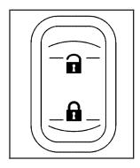
The power door lock switches are located on the driver's and front passenger's doors. Press the bottom of the switch to lock all doors. Press the top of the switch to unlock all doors.
